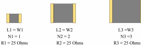
• Resistor value = sheet resistivity x ratio of element length to width ( $R = Rs \times L/W$ )
