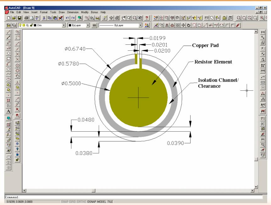
▲ Draw 7 – 1K ohm resistor design (heater).
