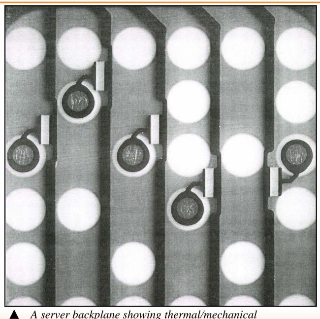
A server backplane showing thermal/mechanical isolation of OhmegaPly® resistors
