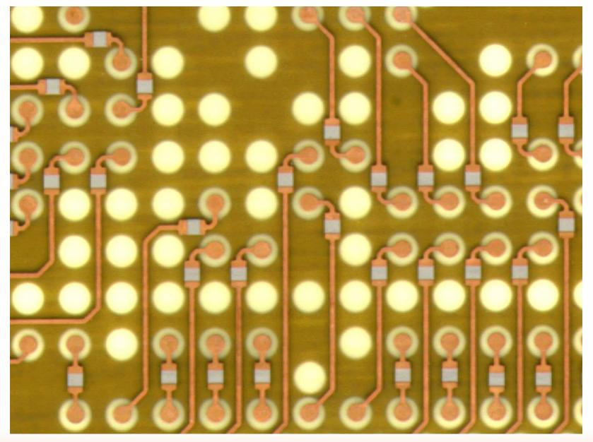
Series termination resistors for telecom switching card
