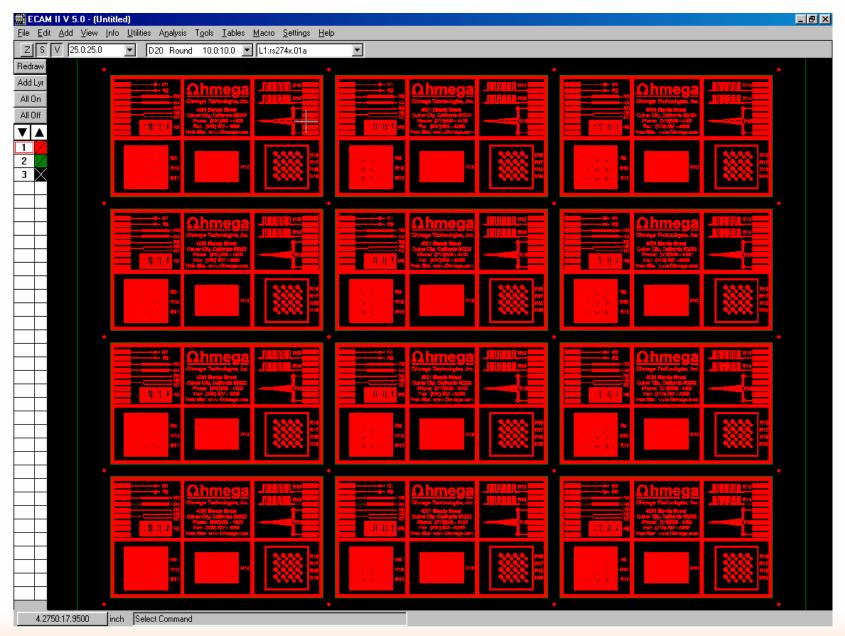
**ECAM** Panelized PCB - copper
