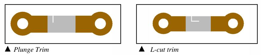
The top figures are designed without special modification for trimming except to provide enough area to handle power dissipation and current if cross-section is reduced by a conventional trim cut
