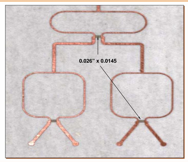
Enlargement of a four-up array 16-way power divider with 50 Ω/sq OhmegaPly<sup>®</sup> resistors
