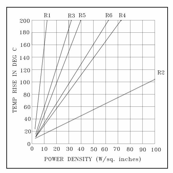
Because the resistor is buried within the layers, the physical and thermal characteristics of the substrate directly affect the manner of heat dissipation from the substrate e.g. the thickness of the substrate and cladding (heat sinking effect). As shown in the above graph the temperature rise in the resistor (R1) is improved significantly when copper cladding (R2) is used
