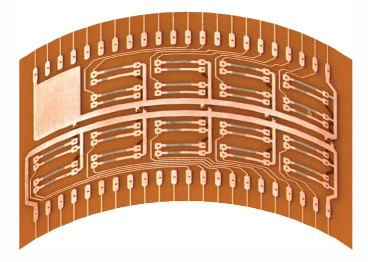
OhmegaPly<sup>®</sup> Resistors in Flex Circuit
