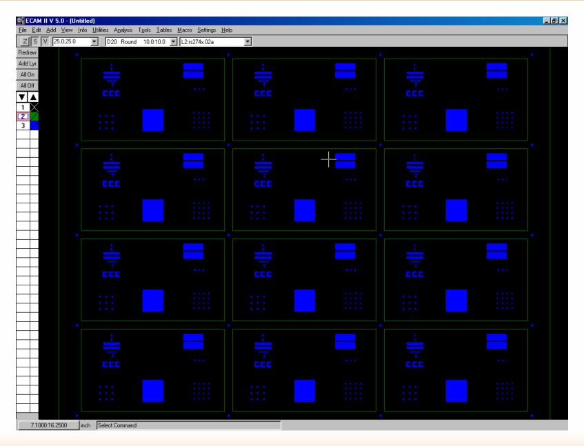
▲ ECAM Panelized PCB - resistor
