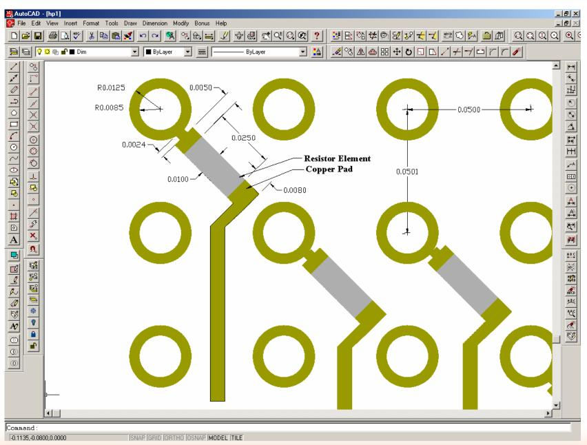
Draw 1 – 62 ohm resistor design under BGA.
