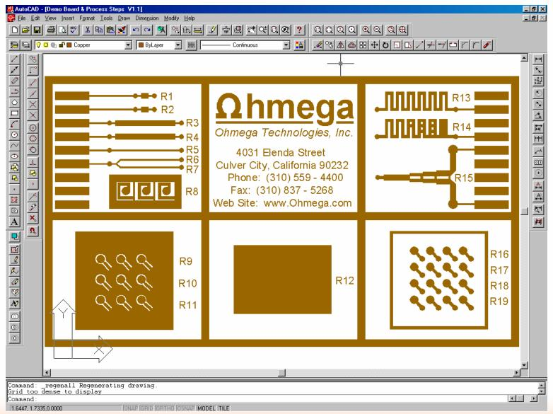
Composite image of conductors and resistors
