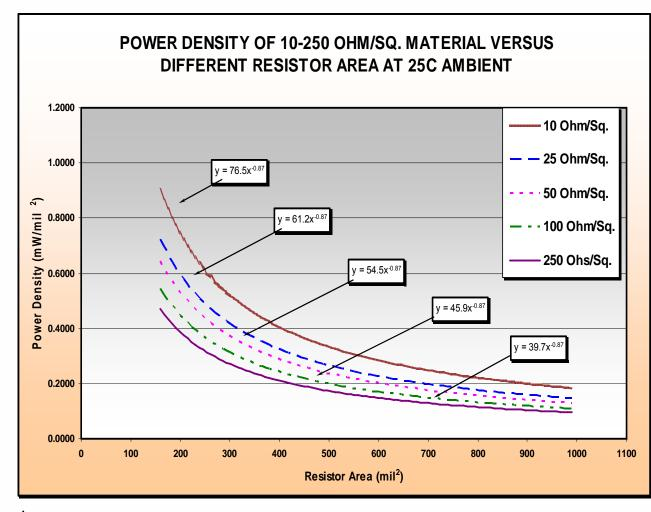
For resistor area larger than 1100 mil<sup>2</sup>, the recommended power dissipation at 25 °C ambient is as follows:
