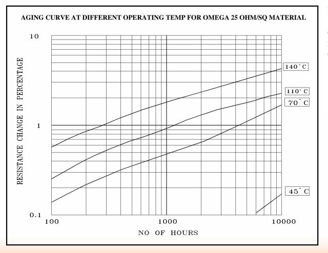
Because the resistor film is a part of laminate, the physical and thermal characteristics of the substrate become major considerations. The heat dissipation of resistor films depends on:
