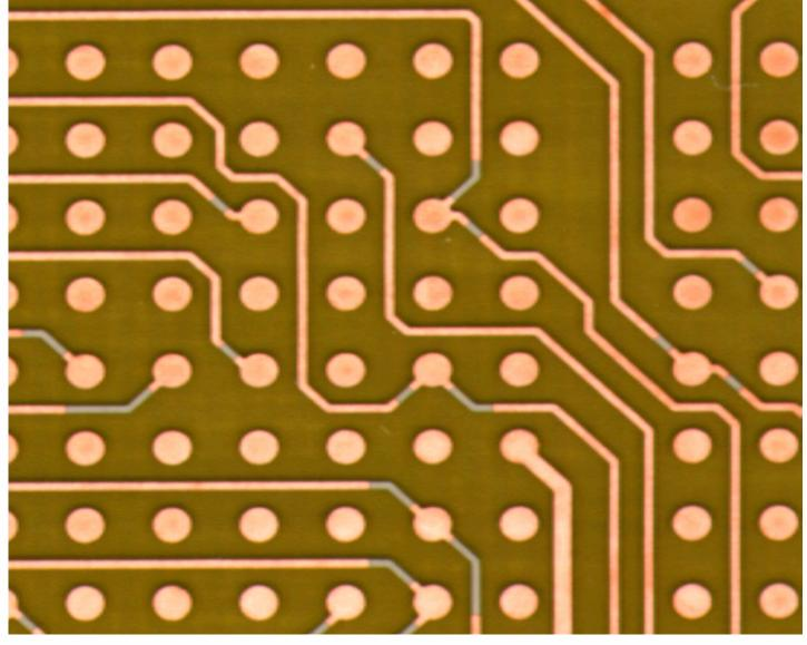
ORBIT<sup>TM</sup> as series terminating resistors.
