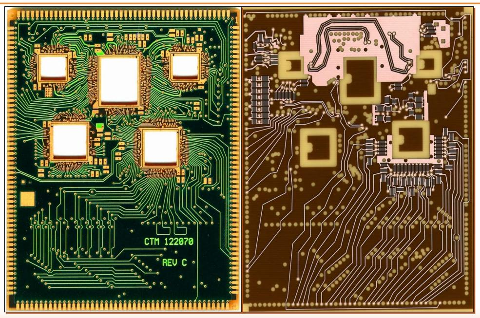
▲ Buried resistor application – 2" X 3" Probe Card.
