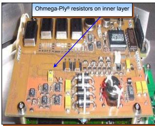
▲ Ohmega-Ply<sup>®</sup> resistors in electronic lander PC board
