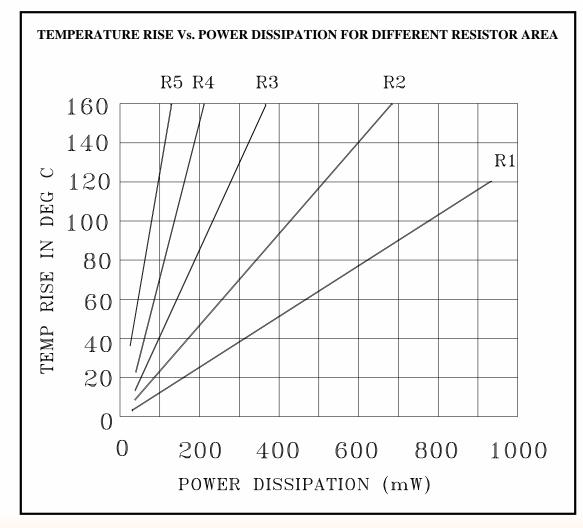
R1 =  $25\Omega$  area of R1 =  $0.500 \ge 0.500 = 0.2500$  in<sup>2</sup> R2 =  $25\Omega$ area of R2 =  $0.250 \ge 0.0625$  in<sup>2</sup> R3 =  $25\Omega$ area of R3 =  $0.125 \ge 0.0125 = 0.0126$  in<sup>2</sup> R4 =  $25\Omega$ area of R4 =  $0.063 \ge 0.0039$  in<sup>2</sup> R5 =  $25\Omega$ area of R5 =  $0.031 \ge 0.0010$  in<sup>2</sup>
