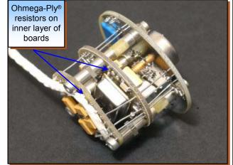
▲ X-Ray Spectrometer (XRS) with Ohmega-Ply<sup>®</sup> resistors
