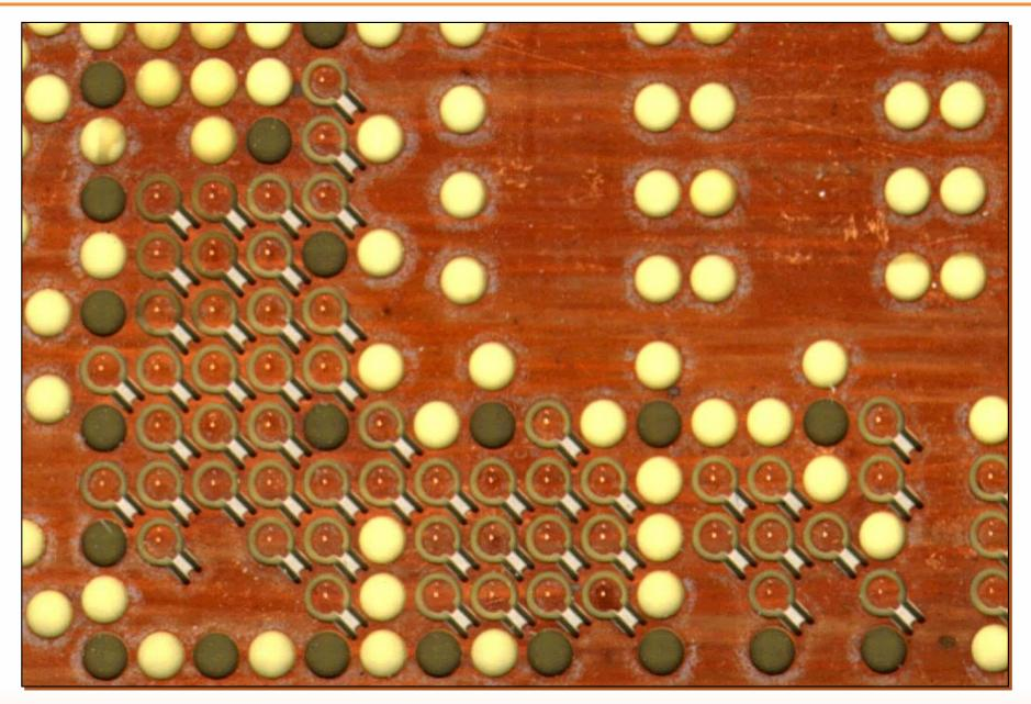
▲ Parallel termination resistors in a BGA package.
