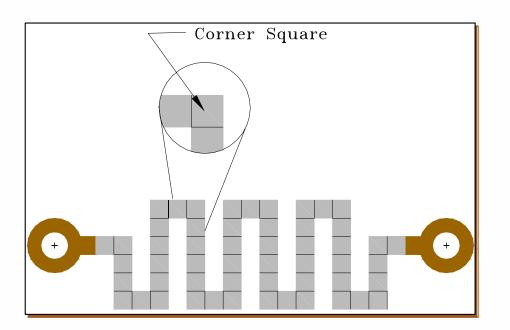
e.g., sheet resistance  $(R_s) = 100 \ \Omega/\Box$ No. of squares = 37 No. of corner squares = 16 Total No. of effective squares = 37 + (16 x 0.56) = 45.9  $\approx 46$ Resistance value = 46 x 100 = 4.6 K $\Omega$
