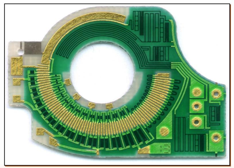
Surface resistor application –Potentiometer (35 mm SLR camera).
