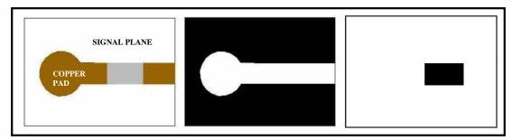
Composite (negative film) conductor protect
